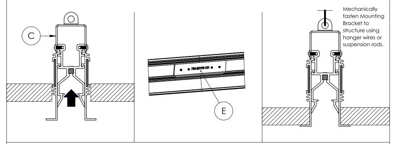
**Step 6; Install Luminaires:** Connect Luminaires (B) to Low Voltage Cables. Then install Luminaires (B) by pushing them up until they snap into Housings (A). If possible, arrange Luminaire (B) lenses so that they overlap fixture joints. Finally, power the Luminaires (B) to double check electrical connections. Completed installation is shown below.
