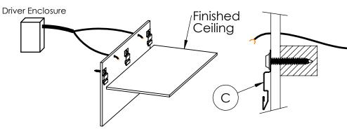
**Step 4; Mounting Hardware:** Install Endcaps on first and last Housing (A) of each run. Install Joiners on each Housing (A), before putting in the ceiling. Install Snap-in Clips onto Luminaire (B) using provided screws.
