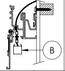
**Step 6; Install Luminaire:** Push the Luminaries (B) up until they snap into the Housings (A). Arrange the Luminaires (B) as close to each other as possible. Next power the Luminaires (B) to double check electrical connections. When the ceiling is installed, it will need to end 2 - 1/2" from the
