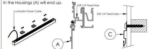
Step 3; Remote Drivers: Install the Remote drivers and run Low voltage cables to the wall. Then run the Low voltage cables through the feed holes drilled above the Mounting Clips (C).
