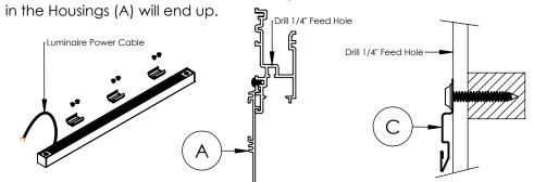
Step 3; Remote Drivers: Install the Remote drivers and run Low voltage cables to the wall. Then run the Low voltage cables through the feed holes drilled above the Mounting Clips (C).
