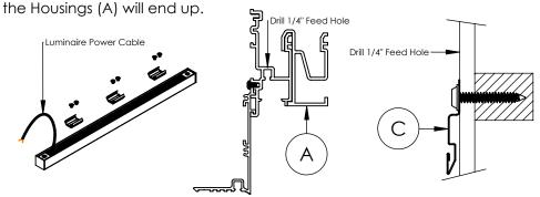
**Step 3; Remote Drivers:** Install the Remote drivers and run Low voltage cables to the wall. Then run the Low voltage cables through the feed holes
