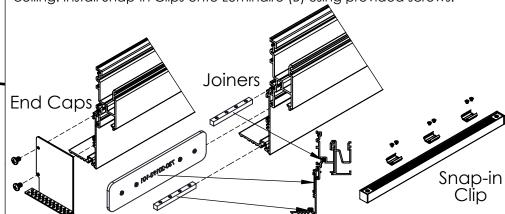
Step 6: Install Luminaire/Plaster: Push the Luminaries (B) up until they snap into the Housings (A). Position Luminaires so that there are no noticeable gaps between them. Next power the Luminaires (B) to double check electrical connections. When the ceiling is installed, it will need to end 2 - 3/4" from the the wall to accomodate the Housings (A). Ensure that the Housing (A) is flush with the ceiling. Once everything is in place and working properly, plaster over the flange as shown below.
