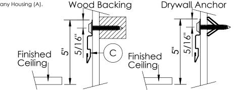
**Step 2; Feed Holes:** Determine which end the Luminaire (B) cables will start at on each Housing (A) and mark them on the shown location on the Housings (A), around 1 inch from the end. Then drill 1/4" holes where you marked. Finally look at where the Housings (A) will be installed and drill 1/4" holes above the line of the Mounting Clips, and close to where the holes in
