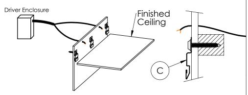
**Step 4; Mounting Hardware:** Install Endcaps on first and last Housing (A) of each run. Install Joiners on each Housing (A), before putting in the ceiling. Install Snap-in Clips onto Luminaire (B) using provided screws.
