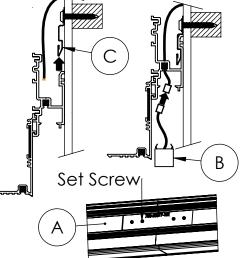
Step 6: Install Luminaire/Plaster: Push the Luminaries (B) up until they snap into the Housings (A). Position Luminaires so that there are no noticeable gaps between them. Next power the Luminaires (B) to double check electrical connections. When the ceiling is installed, it will need to end 1 - 3/4" from the the wall to accomodate the Housings (A). Ensure that the Housing (A) is flush with the ceiling. Once everything is in place and working properly, plaster over the flange as shown below.
