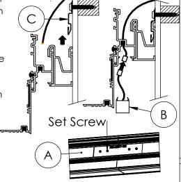
**Step 4; Mounting Hardware:** Install Endcaps on first and last Housing (A) of each run. Install Joiners on each Housing (A), before putting in the ceiling. Install Snap-in Clips onto Luminaire (B) using provided screws.
