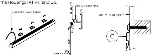
**Step 3; Remote Drivers:** Install the Remote drivers and run Low voltage cables to the wall. Then run the Low voltage cables through the feed holes drilled above the Mounting Clips (C).
