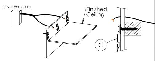
**Step 4; Mounting Hardware:** Install Endcaps on first and last Housing (A) of each run. Then install Joiners on each Housing (A), before putting in the ceiling. Install Snap-in Clips onto Luminaires (B) using provided screws.
