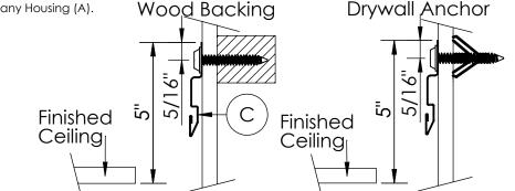
**Step 2; Feed Holes:** Determine which end the Luminaire (B) cables will start at on each Housing (A) and mark them on the shown location on the Housings (A), no less than 3 inches from the end. Then drill 1/4" holes where you marked. Finally look at where the Housings (A) will be installed and drill 1/4" holes above the line of the Mounting Clips, and close to where the holes
