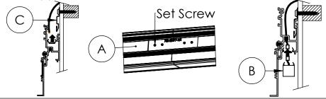
Step 6: Install Luminaire: Push the Luminaries (B) up until they snap into the Housings (A). Position Luminaires so that there are no noticeable gaps between them. Next Power the Luminaires (B) to double check electrical connections. When the ceiling is installed, it will need to end 1 - 1/4" from the the wall to accomodate the Housings (A)
