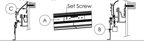
Step 6: Install Luminaire: Push the Luminaries (B) up until they snap into the Housings (A). Position Luminaires so that there are no noticeable gaps between them. Next Power the Luminaires (B) to double check electrical connections. When the ceiling is installed, it will need to end 2 - 1/4" from the
