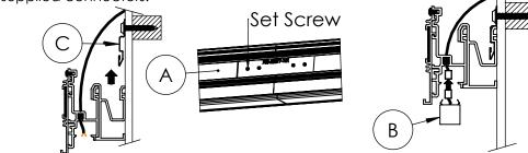
**Step 6; Install Luminaire:** Push the Luminaries (B) up until they snap into the Housings (A). If possible, arrange Luminaire (B) lenses so that they overlap fixture joints. Next, power the Luminaires (B) to double check electrical connections. When the ceiling is installed, it will need to end 2 - 1/2" from the the wall to accomodate the Housings (A).
