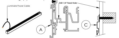
**Step 4; Mounting Hardware:** Install Endcaps on first and last Housing (A) of each run. Install Joiners on each Housing (A), before putting in the ceiling. Install Snap-in Clips onto Luminaires
