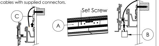
**Step 2; Feed Holes:** Determine which end the Luminaire (B) cables will start at on each Housing (A) and mark them on the shown location on the Housings (A), no less than 3 inches from the end. Then drill 1/4" holes where you marked. Finally look at where the Housings (A) will be installed and drill 1/4" holes above the line of the Mounting Clips, and close to where the holes
