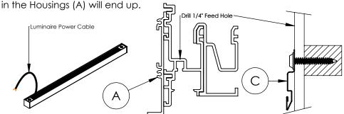
**Step 4; Mounting Hardware:** Install Endcaps on first and last Housing (A) of each run. Insert two T - grid Brackets (D) and Joiners on each Housing (A). T - grid Brackets (D) should be positioned equally spaced from ends of Housing (A), and fastened with provided set screws. Then install Snap-ir
