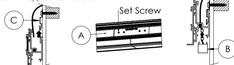
Step 6; Install Luminaire: Push the Luminaries (B) up until they snap into the Housings (A). When the ceiling and grid is installed, it will need to end 1 - 3/4" from the the wall (as shown below) to accomodate the Housings (A). Then fold the Grid Bracket (D) over the T - grid and drive a screw through them both (recommended Phillips #8-32 x 3/8"). Finally power the Luminaires (B) to double check electrical connections.
