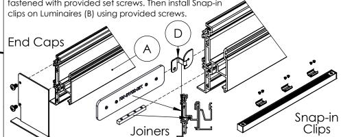
Step 6; Install Luminaire: Push the Luminaries (B) up until they snap into the Housings (A). When the ceiling and grid is installed, it will need to end 2 - 3/4" from the the wall (as shown below) to accomodate the Housings (A). Then fold the Grid Bracket (D) over the T - grid and drive a screw through them both (recommended Phillips #8-32 x 3/8"). Finally power the Luminaires (B) to double check electrical
