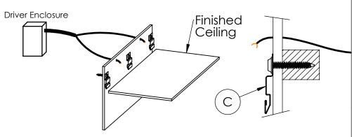
Step 4; Mounting Hardware: Install Endcaps on first and last Housing (A) and Luminaire (B) of each run. Install Joiners on each Housing (A), before putting in the ceiling. Install Snap-in Clips onto Luminaire (B) using provided screws.
