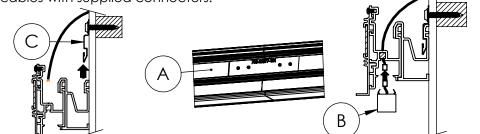
**Step 6; Install Luminaire:** Push the Luminaires (B) up until they snap into the Housings (A). If possible, arrange Luminaire (B) lenses so that they overlap fixture joints. Next, power the Luminaires (B) to double check electrical connections. When the ceiling is installed, it will need to end 2 - 1/4" from the the wall to accomodate the Housings (A).
