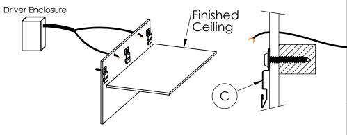
**Step 4; Mounting Hardware:** Install Endcaps on first and last Housing (A) of each run. Then install Joiners on each Housing (A), before putting in the ceiling. Install Snap-in Clips on Luminaire (B) using provided screws.
