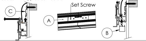
Step 6: Install Luminaire: Push the Luminaires (B) up until they snap into the Housings (A). If possible, arrange Luminaire (B) lenses so that they overlap fixture joints. Next, power the Luminaires (B) to double check electrical connections. When the ceiling is installed, it will need to end 1 - 1/4" from the the wall to accomodate the Housings (A).
