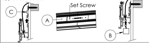
**Step 6; Install Luminaire:** Push the Luminaries (B) up until they snap into the Housings (A). If possible, arrange Luminaire (B) lenses so that they overlap fixture joints. Next, power the Luminaires (B) to double check electrical connections. When the ceiling is installed, it will need to end 1 - 1/2" from the the wall to accomodate the Housings (A).
