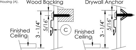
**Step 2; Feed Holes:** Determine which end the Luminaire (B) cables will start at on each Housing (A) and mark them on the shown location on the Housings (A), no less than 3 inches from the end. Then drill 1/4" holes where you marked. Finally look at where the Housings (A) will be installed and drill
