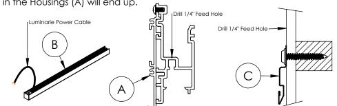
Step 3; Remote Drivers: Install the Remote drivers and run Low voltage cables to the wall. Then run the Low voltage cables through the feed holes drilled above the Mounting Clips (C).
