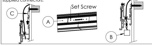
**Step 6; Install Luminaire:** Push the Luminaries (B) up until they snap into the Housings (A). If possible, arrange Luminaire (B) lenses so that they overlap fixture joints. Next, power the Luminaires (B) to double check electrical connections. When the ceiling is installed, it will need to end 1 - 1/2" from the the wall to accomodate the Housings (A).
