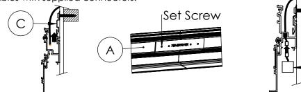
**Step 6; Install Luminaire:** Push the Luminaries (B) up until they snap into the Housings (A). Arrange Luminaires (B) so that there are no noticeable gaps between them. Next power the Luminaires (B) to double check electrical connections. When the ceiling and grid is installed, it will need to end 1 - 3/4" from the the wall (as shown below) to accomodate the Housings (A). Finally fold the Grid Bracket (D) over the T-
