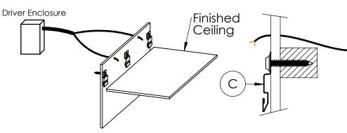
**Step 4; Mounting Hardware:** Install Endcaps on first and last Housing (A) of each run. Insert two T - grid Brackets (D) and Joiners on each Housing (A). T - grid Brackets (D) should be positioned equally spaced from ends of Housing (A), and
