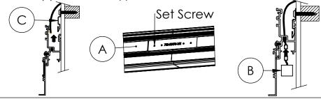
Step 6: Install Luminaire: Push the Luminaries (B) up until they snap into the Housings (A). Position Luminaires so that there are no noticeable gaps between them. Next Power the Luminaires (B) to double check electrical connections. When the ceiling is installed, it will need to end 1 - 1/4" from the the wall to accomodate the Housings (A)
