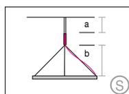
1-point suspension with drivers in pendant canopy PB 366, separate power cable from canopy down. (Up to Ø 1800mm/71")<sup>4</sup>
