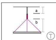
1-point suspension with drivers in pendant canopy PB 366, current-carrying suspension cables from canopy down. (Up to Ø 1800mm/71")<sup>4,5</sup>
