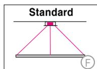
Drivers in center surface mounted canopy (3), current-carrying suspension cables. (Up to Ø 1800mm/71")<sup>4,5</sup>
