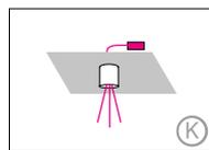
Suspension point as clamping unit with 3 cables and remote technical unit in suspended ceiling.
