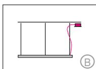
3-point suspension (5m/197" max.) with drivers in offset surface mounted canopy, separate power cable. (Up to Ø 2600mm/102")
