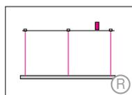
3-point straight suspension (197" max.) with remote mounted drivers, current-carrying suspension cables. (Up to Ø 1800mm/71")<sup>4,5</sup>
