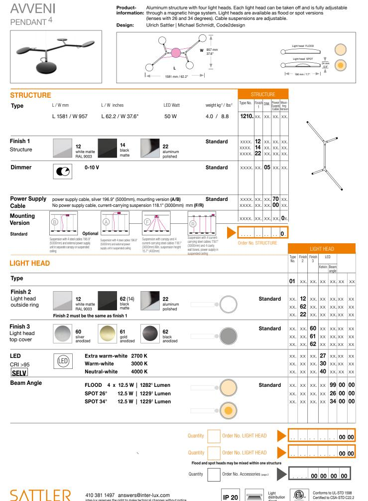
Technical data is subject to change. Errors and omissions excepted 1. Net lumen output: Losses due to diffusors and reflectors are considered. Lumen values refer to an ambient temperature of max. 35° Celsius / 95° Fahrenheit. 2. Weight of lights without remote technical unit or canopy.
