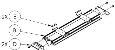
Step 4; Prepare the ceiling and housing for installation: Prepare installation opening by cutting proper size opening on the ceiling. Cut out dimensions are listed below. Drill a 1/4" hole on the surface of housing along centerline of housing 2-1/2" away from one end as shown below.
