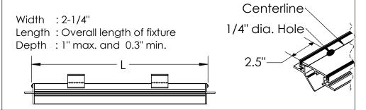
Step 5; Install Joiners: If your order consists of stand alone fixtures, skip this step. If not, connect Housings (B) to each other using supplied Joiner Kits (F). Slide pins into square holes and push Housings (B) together, then center Joiner on joint and drive screws in Joiner as shown below.
