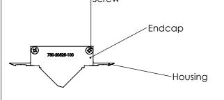
Step 4: The housing should be secured to the backing (wood recommended). In lieu of backing, the housing can be securely mounted to wallstuds and/or anchors as needed. The housing is supplied without mounting holes. These will need to be drilled to align with wood backing, studs or anchors as needed. Use #6 drywall screws. Mark and drill mounting holes in housing in desired locations. (Recommended a max of 24" centers) An alianment aroove is provided to center the hole in the slots.
