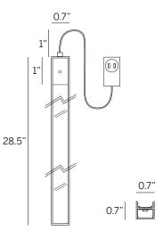
Total Length includes 1" for switch. 1" clearance required for cable.
