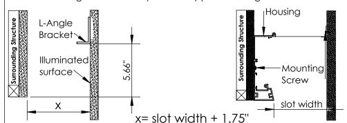
**Grid Ceiling**: Mount L-Angle Bracket to intended illuminated surface at height using appropriate mounting screws at 48" o.c. Mount housing extrusion to the mounting surface using appropriate mounting screws at 16" o.c. Surrounding structure is required to support the weight of the fixture.
