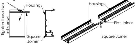
**Step 3:** (If no endcaps skip this step). Install endcaps on first and last housing. Secure by tightening set screws.
