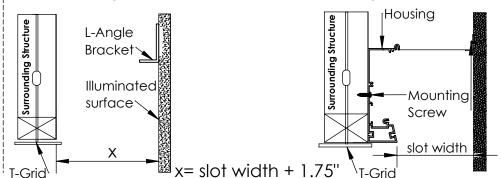
Step 2: (If single housing skip this step) Insert square joiner into next housing, halfway as seen below, secure in place by tightening 2 of the set screws. Insert flat joiner into next housing, place next housing end to end with first housing, slide joiners across housing seam so they are joining both housings. Secure flat joiner by tightening set screws. Mount housing, Repeat until all housing are installed and mounted.
