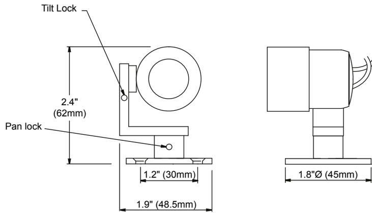
Miniature IP66 adjustable and clamp bracket lockable exterior accent light. Ø 0.8" optics can be changed on site.
