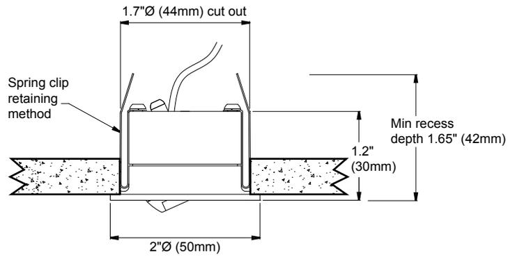
IP66 rated ceiling or panel recessed lockable eyeball fitting that finishes almost flush with the mount surface.
