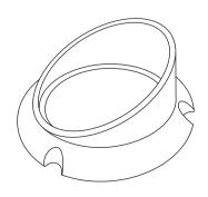
Use the snoot in place of the bezel for additional glare protection.
