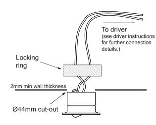
Screw the locking plate down to secure the fitting in position.
