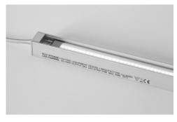
Micro LED strip fitted into 0.65" x 0.65" channel. IP66 rated for exterior use. Channel length up to 6.5ft (2m); strip comes in 1 inch (25mm) increments.
