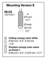
Input voltage for all external power supply units and canopies is 120-277V
