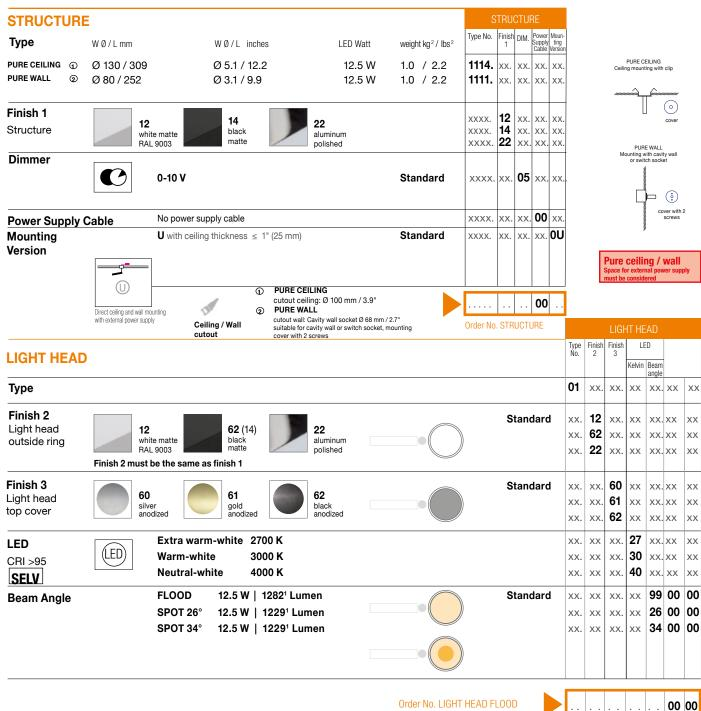
Input voltage for all external power supply units and canopies is 120-277V Remote OT96-D010 driver ordered separately (13.25" (L) x 5" (W) x 2.25" (H))
