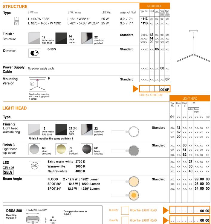
Input voltage for canopies is 120-277V
