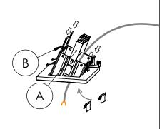
Step 5: Once Housing (A) is flush with the ceiling and secured plaster over the lattice
