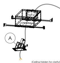
down the Housing (A) into the ceiling using holes in the lattice.
