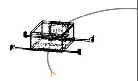
Step 5: Attach the safety cable to the Light Engine (C)(1). Then make the connection between the DC Power wires and Light Engine (C) using the supplied connectors (2).
