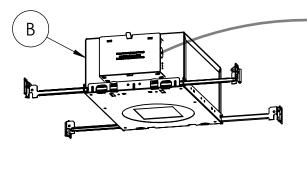
Step 4: Install the ceiling. Make sure that the Housing (B) is flat on top of the ceiling.
