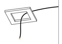
Step 3: Pull AC Power and Dimming Leads through Housing (B). Push Mounting Clips (C) into shown slots until first tabs engage. Then position Housing (B) into hole and push it all the way in
