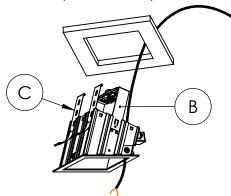
Step 4: Bring Mounting Clips (D) up through the the Housing (B)(1) and push all clips into their respective slots as shown. Make sure that each Clip (C) is pushed down until the Housing (B) is secure in the ceiling (2).
