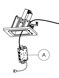
Step 6: Push the Driver (A) up through the Housing (B). Then attach it to the Housing(B), and tighten the thumb screw (2).
