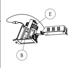
Step 5: Make the connection between the Driver (A) and AC Power/Dimming using the supplied connectors.
