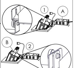
Step 7: Attach the safety cable to the Light Engine (E)(1). Then make the connection between the Driver (A) and Light Engine (E)(2) using the supplied connectors.
