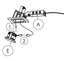
Ceiling Thickness Key Wood Gypsum Material Minimum 1/4" 1/2" 1/16" 1/2" 11/16" Maximum
