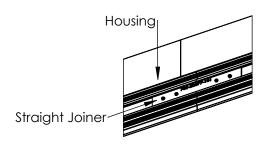
**Step 5:** Feed power cables through feed hole in housing. Install gear trays making electric connections first then insert gear tray into housing. Refer to pages 2&3 for wiring diagrams if needed. Refer to record drawings for gear tray placement. Secure gear tray to housing using screws in pre-drilled holes. If needed, slightly compress sides of housing to properly align gear tray holes with housing. Repeat this step until all gear trays are installed.
