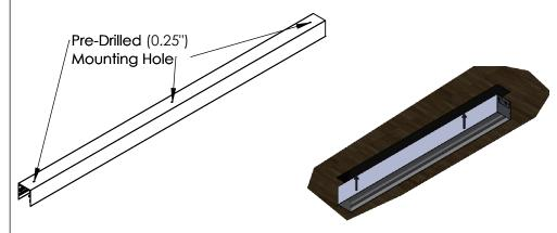
Step 3: (If single housing skip this step) Place one straight joiner on each side of housing as seen below. Tigthen set screws using Allen Key.
