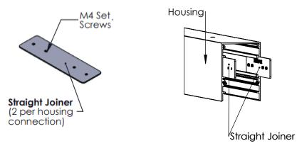
**Step 4:** (If single housing skp this step) Place next housing in ceiling end to end with first housing, slide joiners across housing seam so they are joining both housings. Tighten set screws on joiners. Mount housing. Repeat steps 3-4 until all housing are installed and mounted. Install endcap on last housing as seen in step 1.
