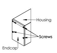
**Step 2:** Mount housing to surface using mounting screws (0.25" diameter pre-drilled holes). Mounting screw must be able to hold weight of the fixture)
