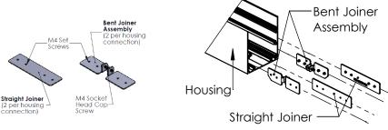
**Step 6:**(If single housing skp this step) Insert airfcraft cable into cable gripper on next housing. Then, slide joiners across housing seam so they are joining both housings. Tighten set screws on joiners, tighten the M4 Cap screw on bent joiners. Repeat steps 5-6 until all housing are installed and leveled. Install endcap on last housing as seen in step 1.
