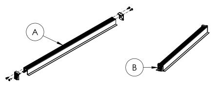
Step 3: Install Grid Brackets: For stand alones, secure Grid Brackets (C) to Luminaire (A), at most 1/2" from ends, using provided screws. For continuous runs, ensure you leave at least 3" at each joint so that Joiners can be installed.
