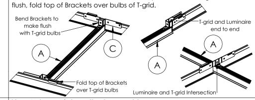
**Step 5; Install Joiners:** If your order consists of stand alone fixtures, skip this step. If not, connect Luminaires (A) to each other using supplied Joiner Kits (D). Slide pins into holes and push Luminaires (A) together, then center Joiner
