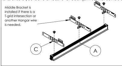
Step 4; Align fixtures with T-grid: Grid Brackets (C) can fold to meet many different arid layouts. Alian Luminaire (A) with T-arid configuration and rest End Caps (B) on the T-grid if possible. Install Joiners (D) (Step 5) as you install a run. Then bend brackets so that they are flush with T-grid bulbs. Once
