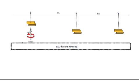
Magnetic Clip - Magnetic clips should already be pre-installed on fixture. Mount fixture directly to magnetic surface.
