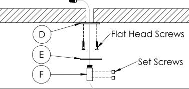
**4C**; Assembly of non-Powered Cable: Follow the same steps above for non-powered suspension cable at the other end of Luminaire (B) except for electrical connection. Level the Luminaire and tighten the plastic set screws on Cable Holder (F).
