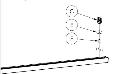
**3D**; Additional Suspension and Power Test: For fixtures longer than 60", install the center suspension the same way described in step 3C. Finally, power and test the Luminaire (B) for proper operation.
