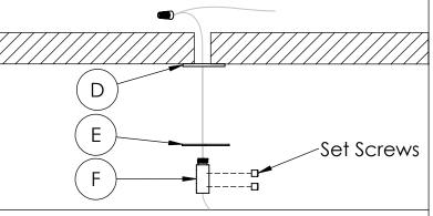
4C; Assembly of non-Powered Cable: Follow the same steps above for non-powered suspension cable at the other end of the Luminaire (B) except for electrical connection. Level the Luminaire and tighten the plastic set screws on Cable Holder (F).
