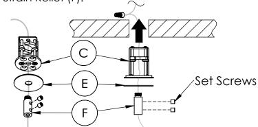
3C; Assembly of non-Powered Cable: Follow the same steps above for non-powered suspension cable at the other end of Luminaire (B) except for electrical connection. Level the Luminaire and tighten the plastic set screws on Cable Holder (F).
