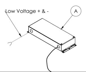
**Step 2**; **Prepare ceiling:** Mark the future position of the fixture on the ceiling. Then, drill holes in ceiling which correspond to suspension method of Luminaire (B). If it is plaster or tile ceiling, cut 1-1/4" holes with hole saw. If it is concrete or wood ceiling, holes should be adequately sized for the suspension cables. Pull low voltage cable of remote driver out through one of the holes.
