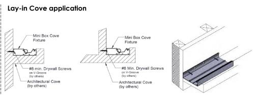
Step 2:(If single housing skp this step) Mount next housing extrusion as shown by sliding the provided joiner into the adjacent housing. Secure in place by tightening set screws. Mount housing to structure. Repeat this step until all housings are installed and mounted.
