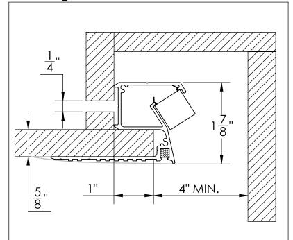
Note: Mini Z-Cove Extrusions are designed to fit around 5/8" drywall.
