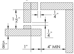
Step 4; Insertion of Housing: Pull low voltage cable through the hole. Align the housing (B) with cantilevered ceiling and insert as shown below.
