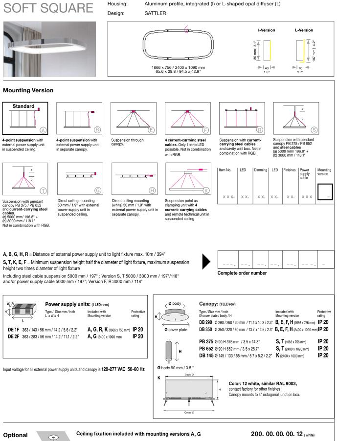
Consisting of a cavity ceiling box with 80 mm / 3.1" round metal cover. Powder coated in white, fine textured. Applicable to mounting version A, G.
