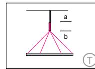
Suspension with pendant canopy PB 366 and current-carrying steel cables.
