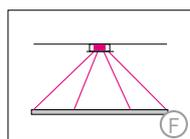
4 current-carrying steel cables. Only 1 strip LED possible. Not in combination with RGB
