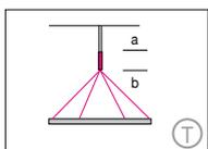
Suspension with pendant canopy PB 366 and current-carrying steel cables. (a) 5000 mm / 196.8" + (b) 3000 mm / 118.1" Not in combination with RGB.
