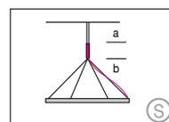
Suspension with pendant canopy PB 366 and steel cables (a) 5000 mm / 196.8" + (b) 3000 mm / 118.1"
