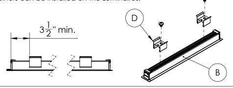
Step 3; Install Spring Clips: For stand alones, secure Spring Clips (D) to Step 4; Prepare the Ceiling for Installation: Prepare installation opening by cutting proper size opening on the ceiling. Cut out dimensions:
