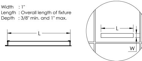
Step 5; Install Joiners: If your order consists of stand alone fixtures, skip this step. If not, connect Luminaires (B) to each other by using supplied Joiner Kits (E). Slide pins into holes and push Luminaires (B) together, then center Joiner on joint and drive screws in Joiner as shown below.
