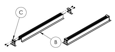
Luminaire (B), at least 3.5" from ends, using provided screws. For continuous runs, ensure you leave at least 3.5" from each end so that joiners can be installed on the Luminaires.
