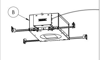
Step 4: Install the ceiling. Make sure that the Housing (B) is flat on top of the ceiling.
