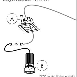
Step 3: Pull DC Power wires through Housing (B).
