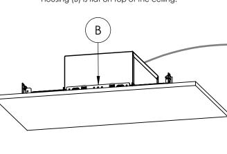
Step 5: Cut ceiling hole that matches the position and dimensions of the Construction Plate (B) hole.
