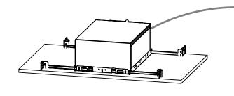
Step 4: Position Housing (A) into ceiling/Plenum hole.
