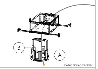
Step 6: Push the Light Engine (D) up into the Housing (A) until it locks into the spring latch as shown.
