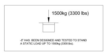
THIS PRODUCT MUST BE INSTALLED IN ACCORDANCE WITH THE APPLICABLE INSTALLATION CODE BY A PERSON FAMILIAR WITH THE CONSTRUCTION AND OPERATION OF THE PRODUCT AND THE HAZARDS INVOLVED
