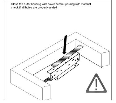
Caution when pouring material around the outer housing (which is set properly). Don't pour the material directly on the upper side of the outer housing. Check if all holes are properly sealed.
