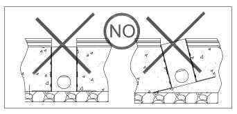
Once the outer housing has been installed the upper edge should not protrude from the floor level
