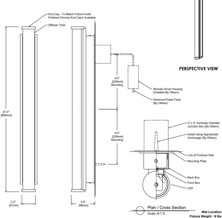
1740WL w 27 М 830 U s SA 19 Options Size Wattage Color Temp Voltage Control Diffuser Finish Model Type EC - Chrome End Caps W - Wall 27" 1 - 120 VAC only 830 - 3,000K SA - Satin Clear Acrylic 19 - Painted Anodized Aluminum -
